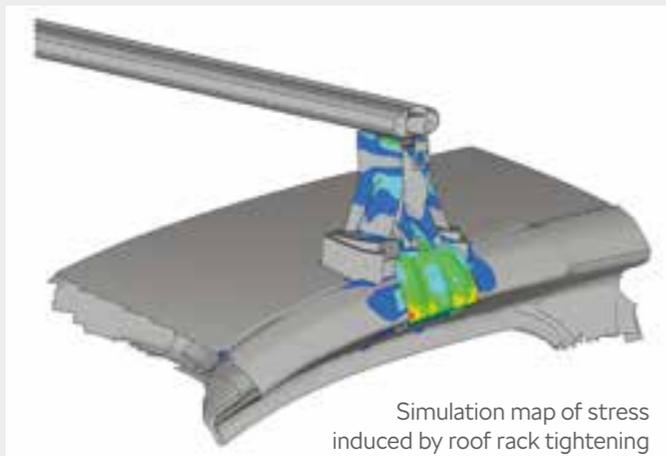
The racks undergo a number of demanding tests. Their resistance to corrosion, loading capacity, strength and durability are tested in various conditions, as well as the subsequent water tightness of the car after their installation. During the so called City Crash test, a rack loaded with 90 kg must remain on the car body under a force of approximately 12 G lasting for 50 milliseconds (impact simulation).
