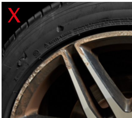
Excessive Damage to wheels
